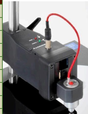
**Type A-D and F-H are user adjustable in the range 60g-150g and supplied at**
