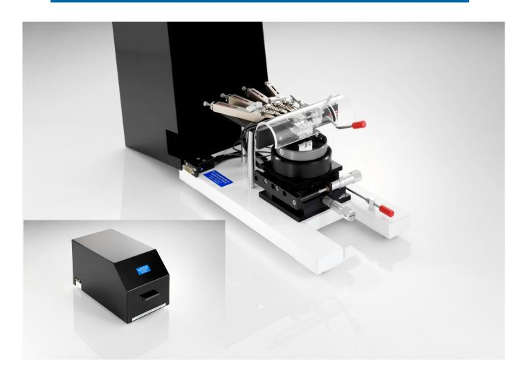
**Jandel Engineering Limited** offers the Universal Probe for use in making both four point probe measurements and 3-point spreading resistance measurements. The maximum sample size is 76mm.
