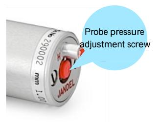
The ranges are: 10-30g, 30-60g, and 60-150g. Within a range the load is adjusted by turning the pressure adjustment screw clockwise. The load indicator goes clockwise from 'L' (low load) round to 'H' (high load).
