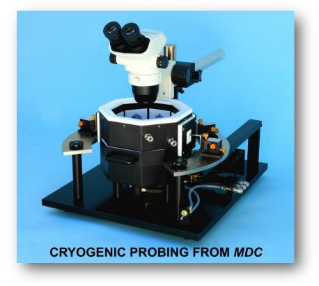
The MDC **Cryogenic Probing System**, Model 441, provides a shielded, electrically quiet, atmosphere controlled environment for high sensitivity capacitance and current measurements at near liquid nitrogen temperatures, 77°K.
