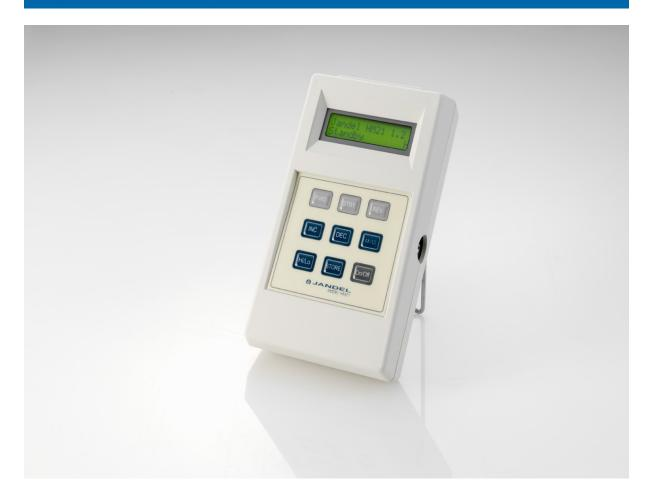
Jandel Engineering Limited offers the HM21 for use in making four point probe measurements. The HM21 has six constant current settings between 100nA and 10mA, and measures voltages from 0.01mV to 1250mV.
